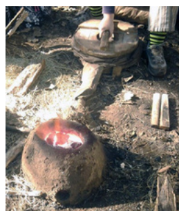
Fig 1. Iron-making experimental bowl furnace utilizing charcoal
